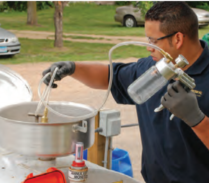
4. Be sure to collect the sample from the bottom of the tank.
