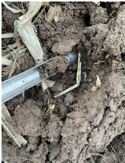
Figure 2 - 2 inches of soil in probe.
