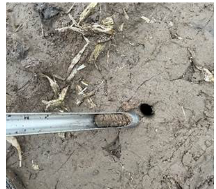
Figure 4 - 3 inches of soil in probe, taken in compacted tire track.
